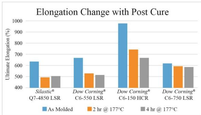
In the third and final figure, elongation is compared in the same manner as previously described. As in each of the previous figures, the new *Dow Corning* C6-750 Liquid Silicone Rubber remains essentially unchanged after post cure whereas the older silicone materials continue to exhibit a fair amount of variability in this measured property as well.
