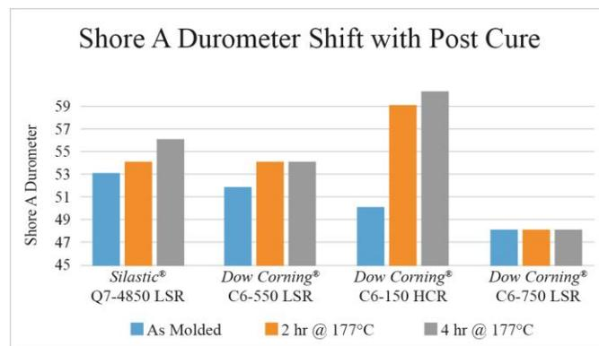
In Figure one, above, the hardness measured for various high and low consistency silicone materials with nominal 50 Shore A hardness are compared as molded, and after a two- and four-hour post-cure at 177°C. The new *Dow Corning*<sup>®</sup> C6-750 Liquid Silicone Rubber is the only material that shows no change in hardness after each post-cure cycle when compared against
