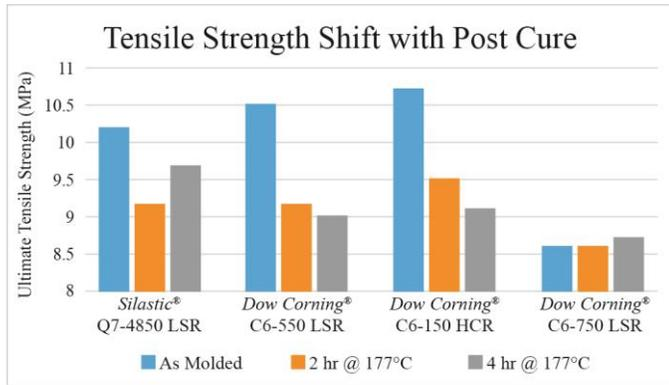
In Figure 2, a comparison of ultimate tensile strength is shown as molded and after the same two-and four-hour post cure that was described above. Again, the new *Dow Corning* C6-750 Liquid Silicone Rubber is essentially unchanged after post cure whereas the older silicone materials exhibit a fair amount of variability in the measured property.
