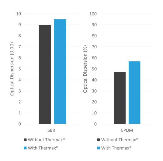
The large particle size of thermal black (avg. 280nm) creates a "ball-bearing" effect that improves the dispersion of other materials into the mix
